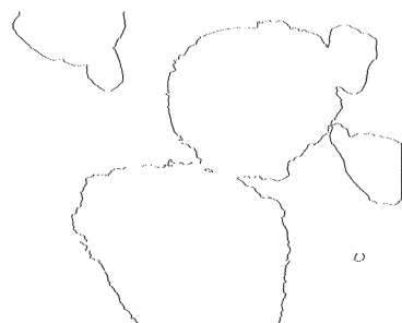
Fig. 2 Edge image which has twin-point structure (pick-up image used line-by-line scan)
